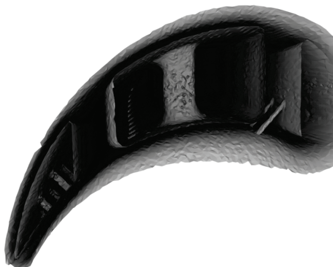
Fig. 3. Mesh created by extracting isosurfaces from volumetric neutron scattering data of turbine blade. Custom software was used to extract and reduce the number of polygons in the mesh.
