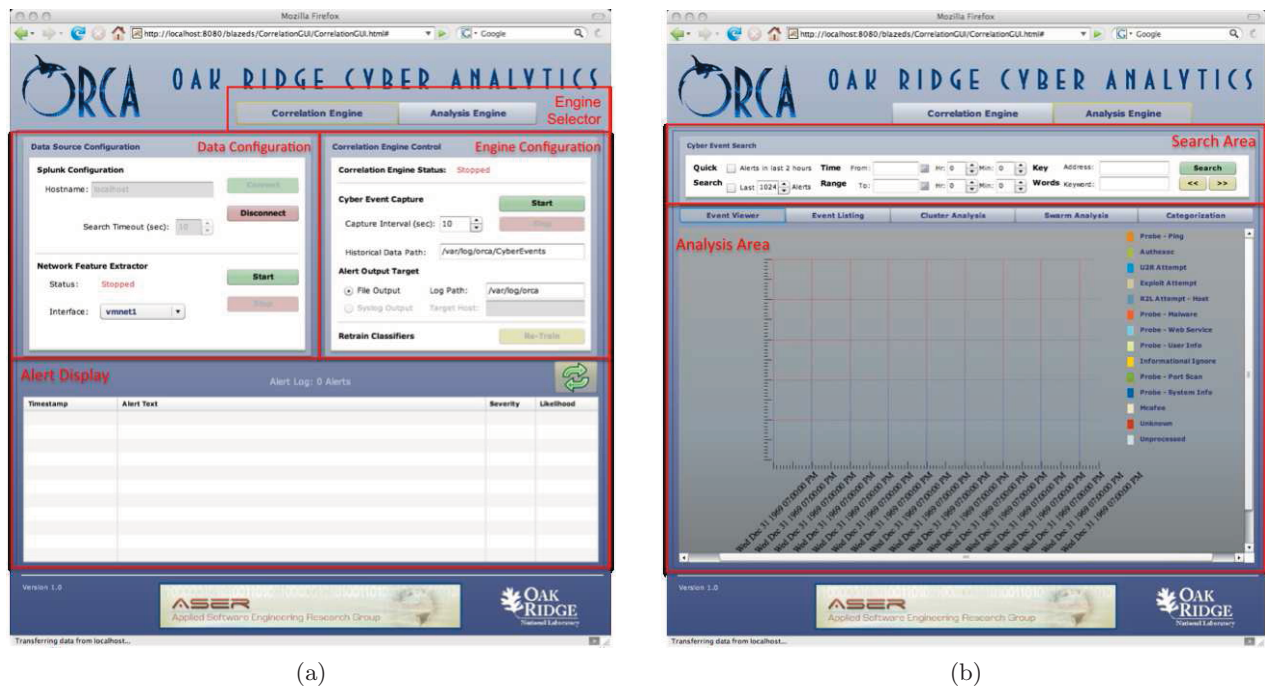
Figure 1. The ORCA Correlation Engine (a) configuration view provides access to the Engine Selector, Data Configuration, Engine Configuration, and Alert Display. The ORCA Analysis Engine (b) configuration view gives the analyst the ability to specify a range of events in the Search Area. This view also provides an Analysis Area toolbar that shows the available analysis methods for the retrieved data.
