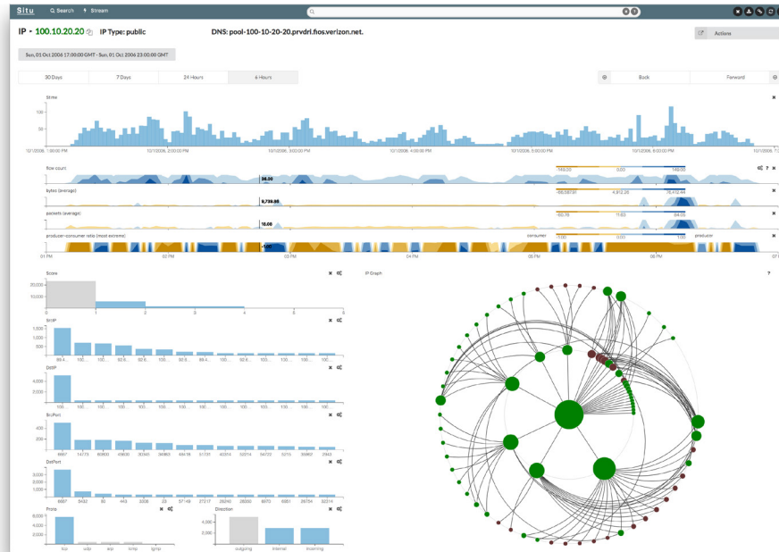
Fig. 1. The IP Detail Page of the Situ system includes a temporal histogram for selecting a time range, horizon graphs for temporal context, bar charts of field distributions for network flows of that IP, and a two-hop communication graph.
